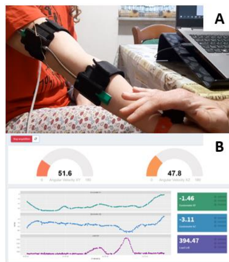
Fig. 5. AUTOMA 2.0 for the upper limb. Motor task performed with an operator (Panel A), and logging of the main displacement, acceleration, and force measurements (Panel B) for the estimation of an objective NMD score.
